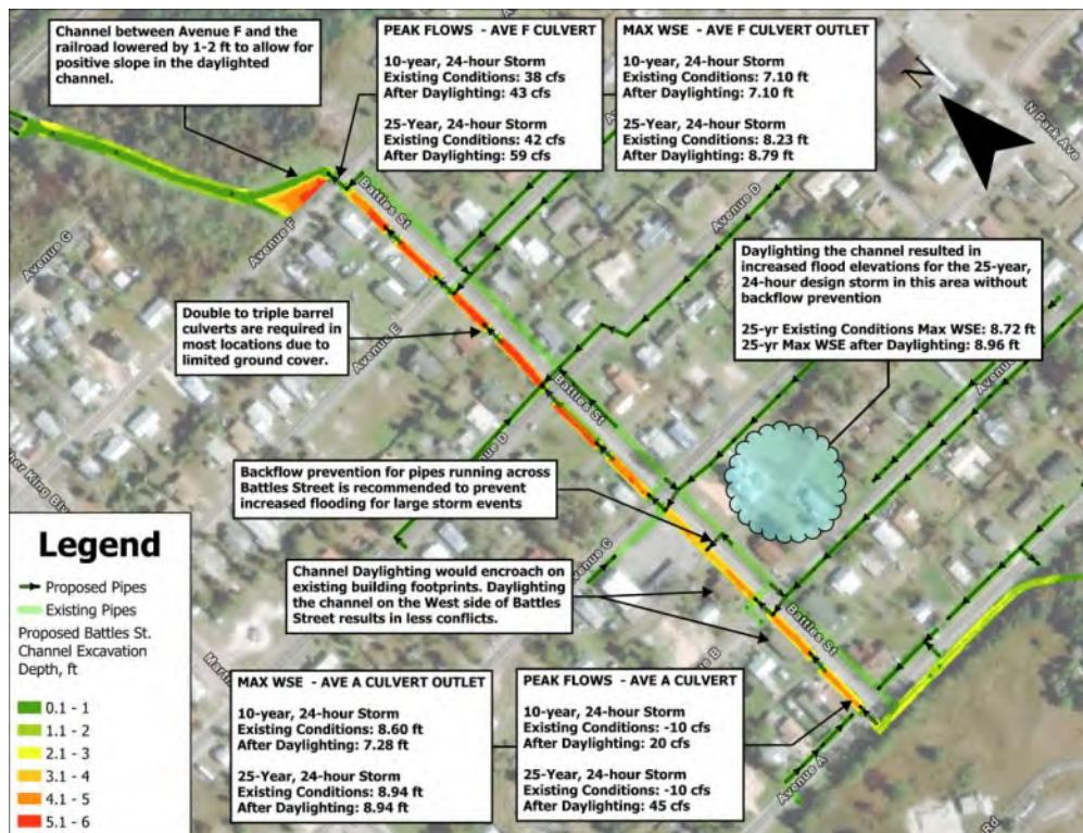
Figure 15: Battles Street Daylighting and Channel Improvements Between Avenue F and The Railroad
