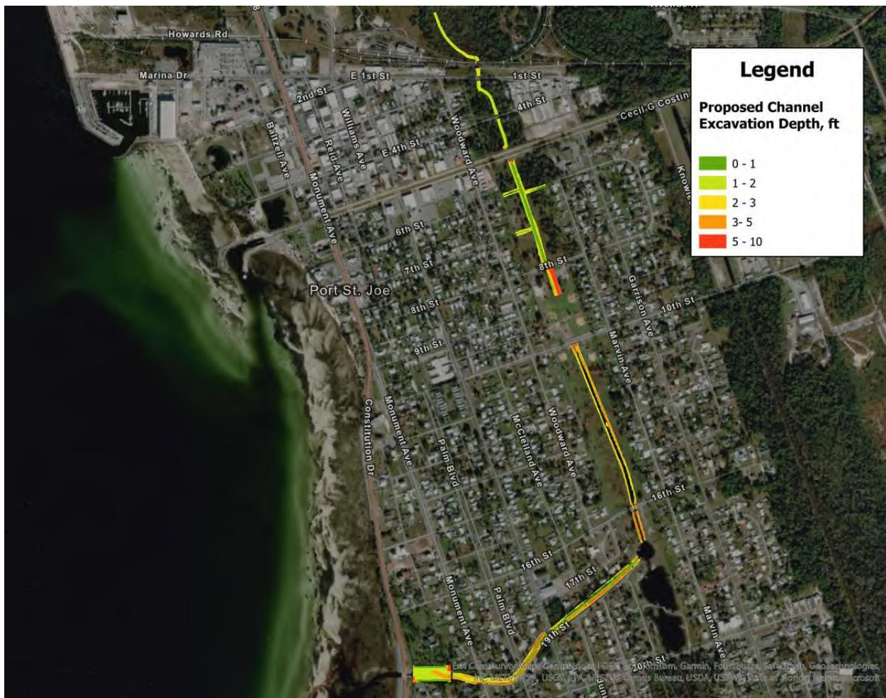
Figure 11: Channel Widening Between 16th and 10th Street
