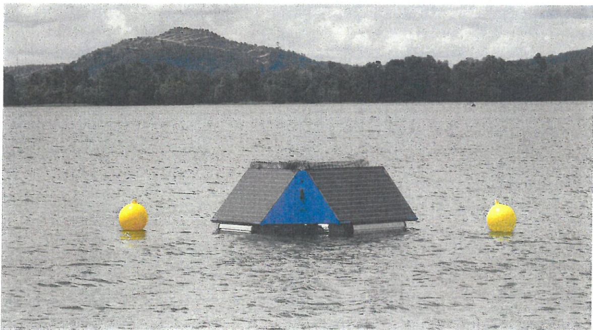
Ultrasonic waves target gas vesicles in the algae, causing them to become less buoyant and sink.
